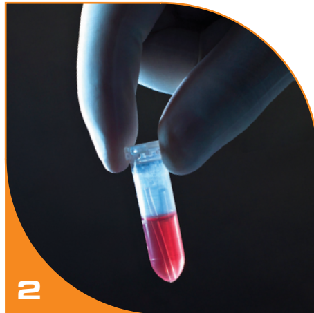
2 Place capillary into tube and invert until mixed.
