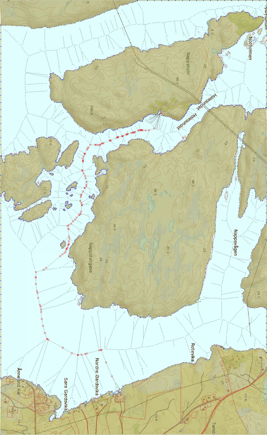
Figure 6.4: The second step involves choosing the waypoints which give the shortest piecewise-linear path.
