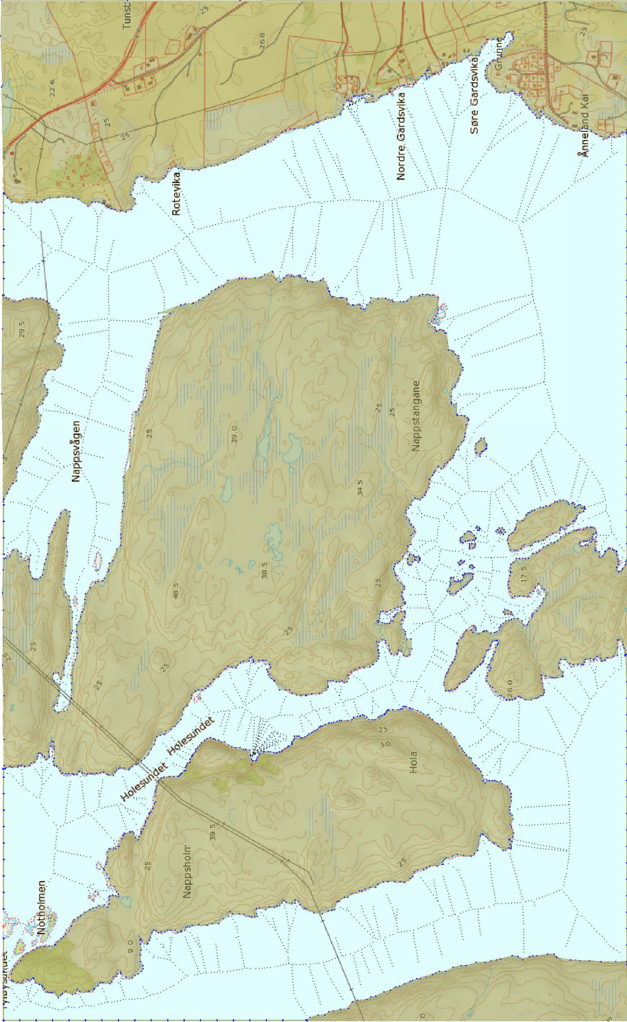
Figure 6.3: The first step involves generating the Voronoi diagram after the obstacles have been defined on the map.
