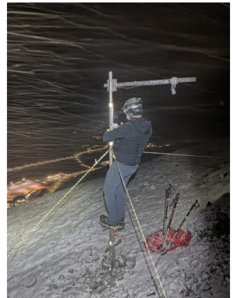
Installation of snow sensor at Gruvefjellet (Photo: H.Hancock)
