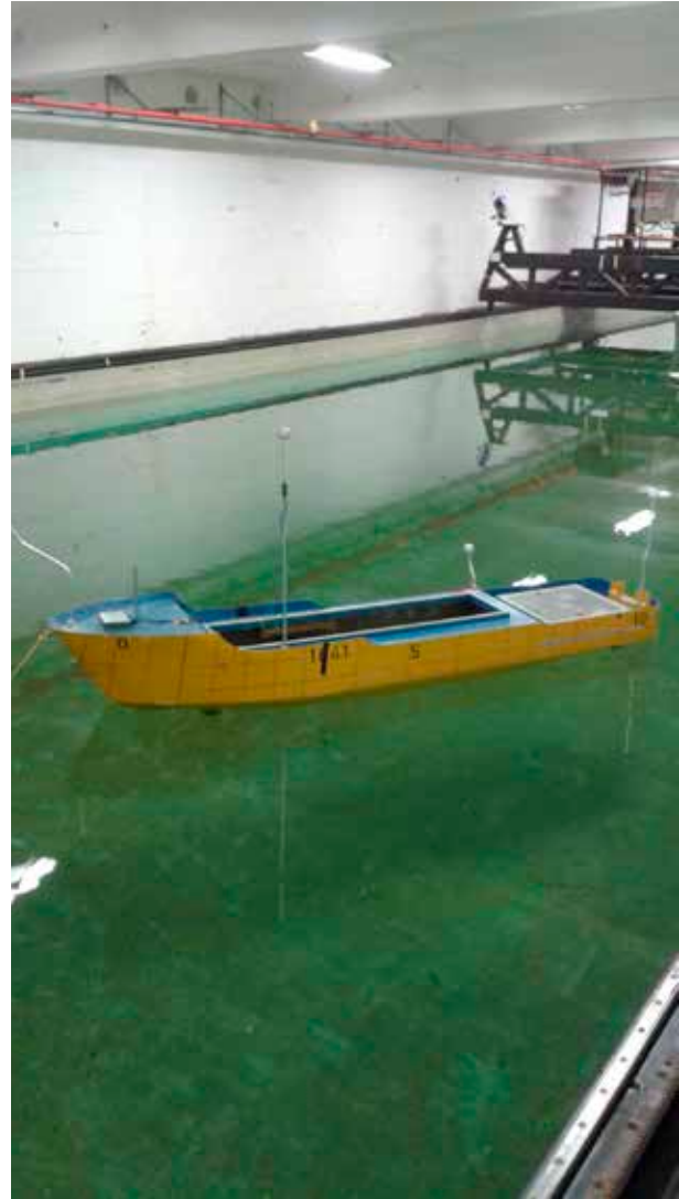
Figure 18 (Astrid H. Brodtkorb, NTNU): New methods for sea state estimation using the ship as a wave buoy is tested with Cybership 3.
