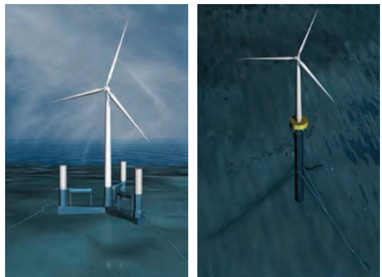
Figure 12: The SFC (to the left) and the STC concepts for converting wind and wave power into electric power, developed at CeSOS, NTNU.
