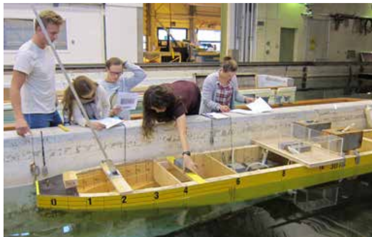
Figure 1: (Kristin Lauritzsen, NTNU): Master students conducting experiments in the towing tank.
