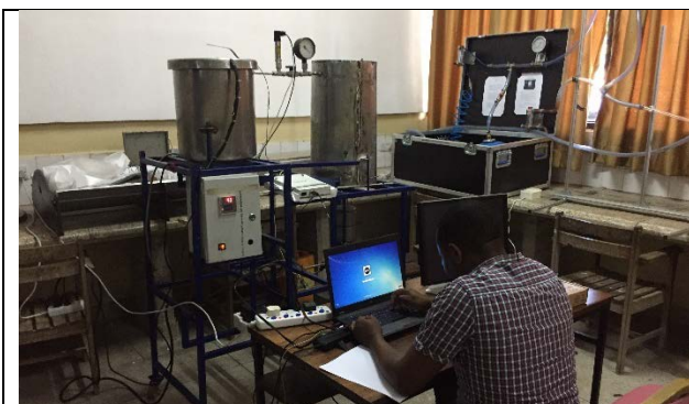
Picture: Adsorption based refrigeration cycle test setup. UDSM
