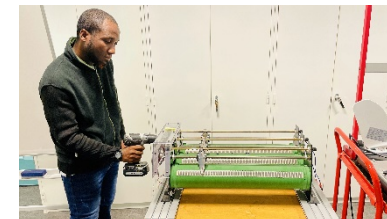
Varying load on the generator
