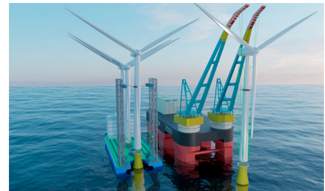
Assembly of offshore wind turbines using a low lifting mechanism compared to traditional lifting technology.
