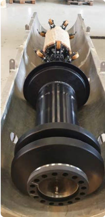
Halfwave / NDT-Global assembly and testing of the newly developed crack detection tool for 20–24" gas pipelines. Photo: Halfwave/NDT-Global.
