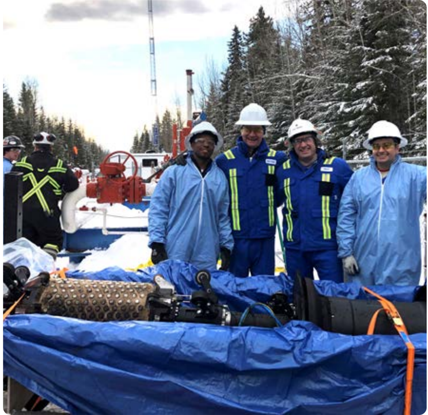
Halfwave / NDT-Global assembly and testing of the newly developed crack detection tool for 20–24" gas pipelines. Photo: Halfwave/NDT-Global.
