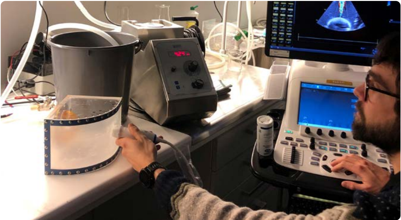
The jet flow phantom for heart valve leakage quantification operated by Postdoctor Stefano Fiorentini. The fluid chamber is shown in the lower left corner, receiving hydrostatic pressure from an elevated bucket. Photo: Hans Torp/NTNU.
